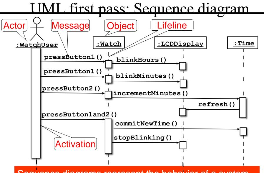
Sequence diagrams represent the behavior of a system as messages ("interactions") between *different objects*
