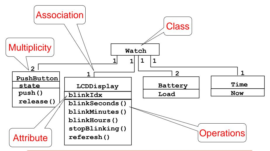
Class diagrams represent the structure of the system
