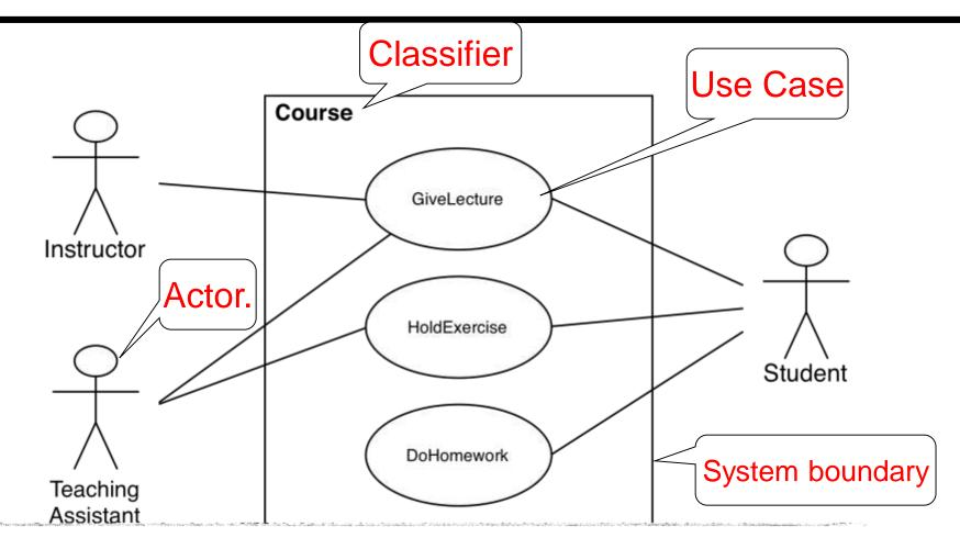
Use case diagram represent the functionality of the system from user's point of view
